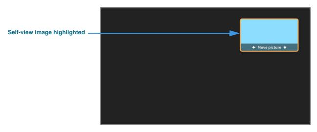
Step 3. Use the arrow keys on the remote control to move the Self-view image down to the bottom-right corner of the screen as shown below.
